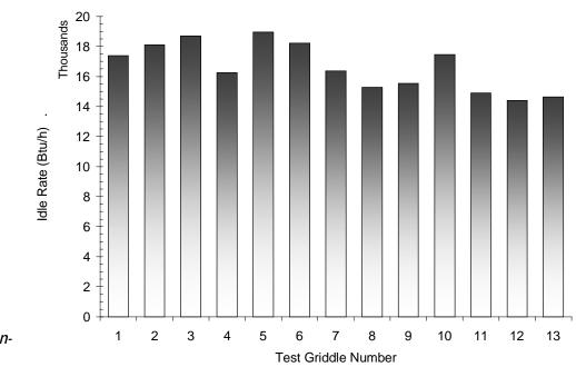
Figure 3-10. 3-ft. gas griddle idle energy rates.
