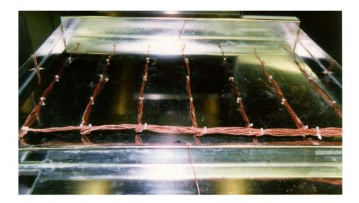
*Figure 3-8. Welded thermocouples to a griddle surface.*
