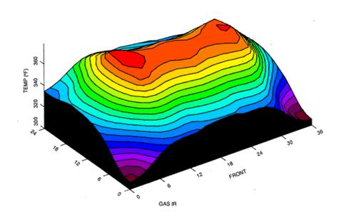
*Figure 3-9. Griddle temperature uniformity plot.*
