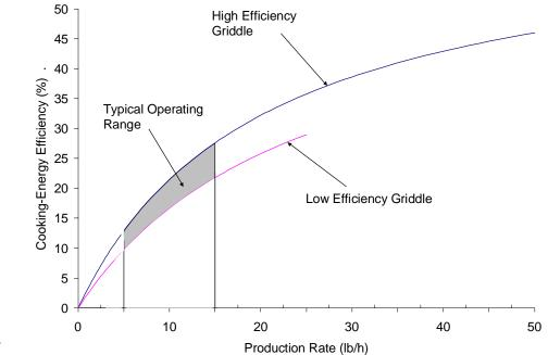
Figure 3-14. Gas 3-ft. griddle cooking-energy efficiency characteristics.
